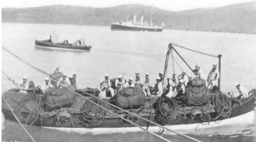
The difficulty of rigging launches to run lines of countermines at night is clear from this photograph of a RN ships' launch in 1896. Also note the low freeboard and the lack of protection for the crew, mines and cables from gunfire.
